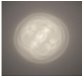
Spot From Collimated Light (no diffuser)
